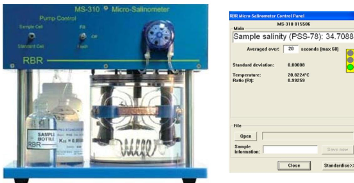
Figure 2 A view of the MS-310 and the software control panel.
