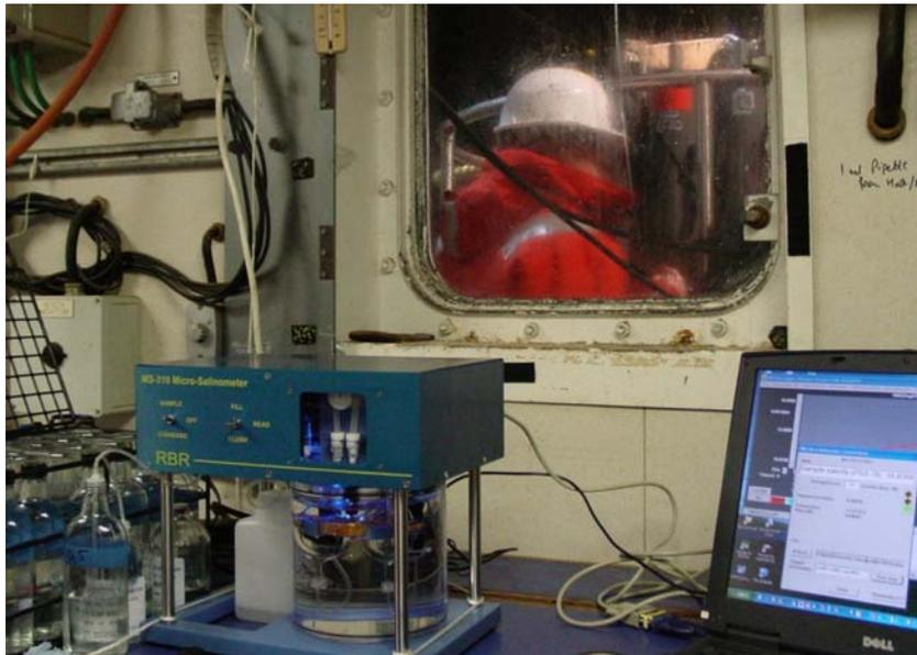
Fig.3. Micro-Salinometer MS-310 in the cold wetlab onboard RRS "Discovery". This places the instrument where it should be – right next to the deck with the sample bottles.
