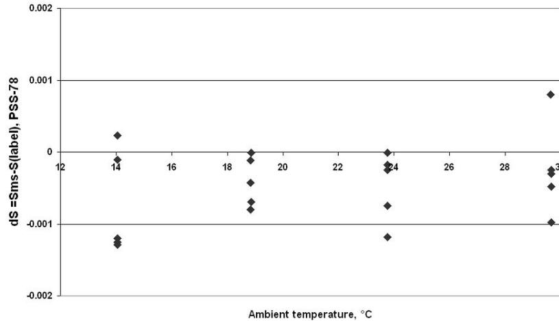
Fig.1 Variation of the measurement of Standard Seawater Salinity with Ambient Temperature. The MS-310 can operate with specification over a wide range of ambient temperatures.
