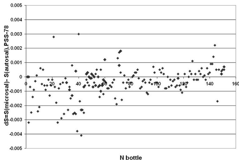
Fig.2. Observed differences between the Micro-Salinometer MS-310 and Autosal 8400B on a set of samples taken during the RRS "Discovery" Cruise 298.
